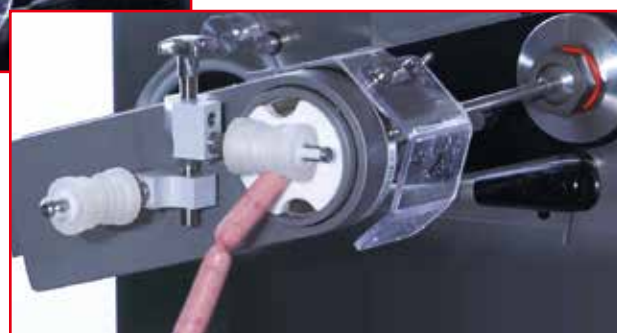
Stuffing of collagen and cellulose casing
